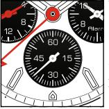
When the battery nears its end, the small second hand moves at two-second intervals instead of the normal one-second intervals. In that case, have the battery replaced with a new one as soon as possible.
