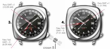
3. Unscrew the crown B & put it into position 2. Turn this crown B anticlockwise to set the GMT hand at the desired second time zone.
